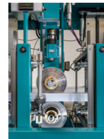
Machine for crimping heat-insulated profiles
